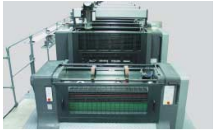
Fig. A13 In-line varnishing unit with extended drying
