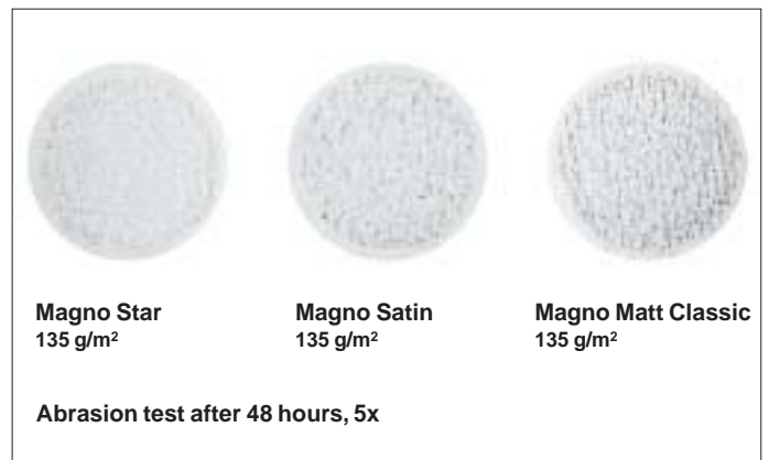
Fig. A11 For comparison, the paper surfaces illustrated above after the abrasion test according to Fogra specifications.
